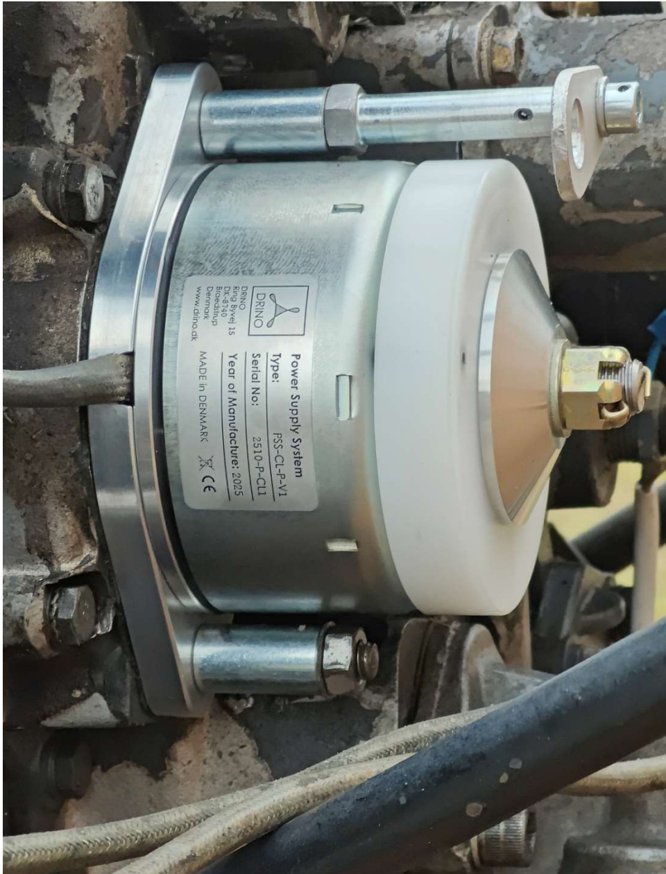
PSS-CL-P-V1 during installation on a Lycoming O-360
